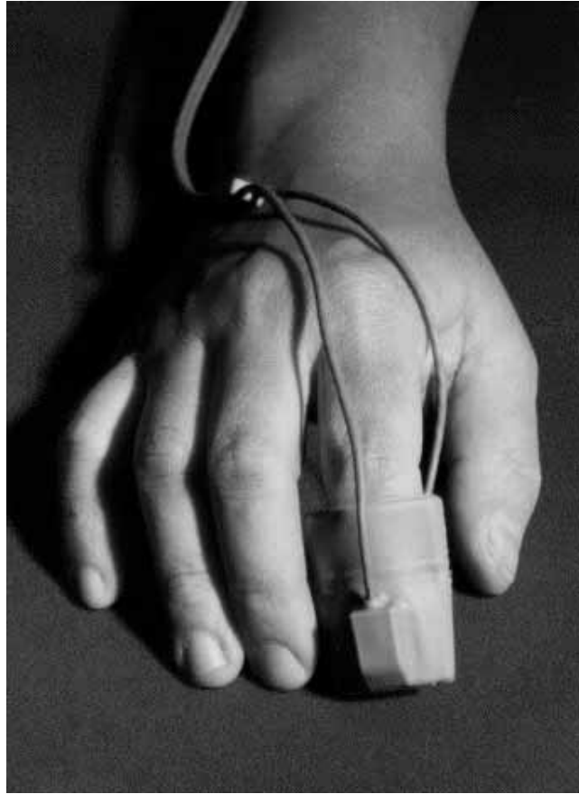
Fig. 12. The HP M1192A pediatric sensor has a closed housing to shield it from interfering ambient light.
